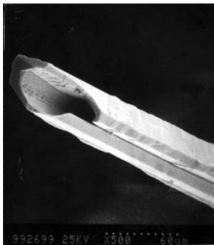
Fig. 10 SEM image of a single selenium tubular crystal obtained from ethanol, showing an uniform crevice running along the c axis.
